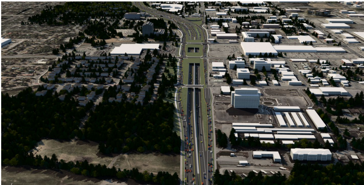
Figure 50: Multi-Interchange Concept – Variant 2 (Loop Ramp) looking south with covers over the depressed freeway section
