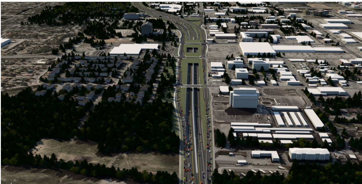
Figure ES-7: Multi-Interchange Concept – Variant 2 (Loop Ramp) looking south with covers over the depressed freeway section
