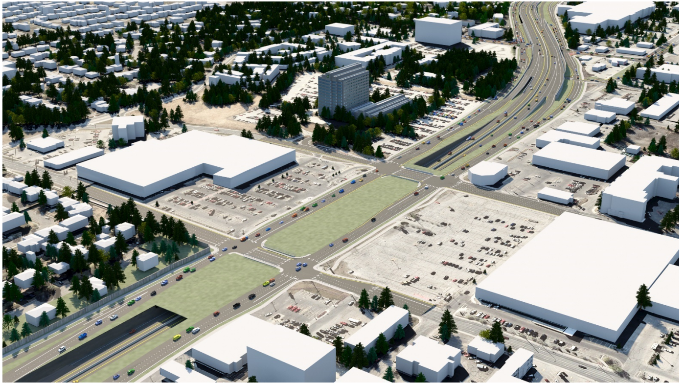
Figure 47: Multi-Interchange Concept – Variant 1 (Median U-Turn) looking south-east with a cover over the depressed freeway section
