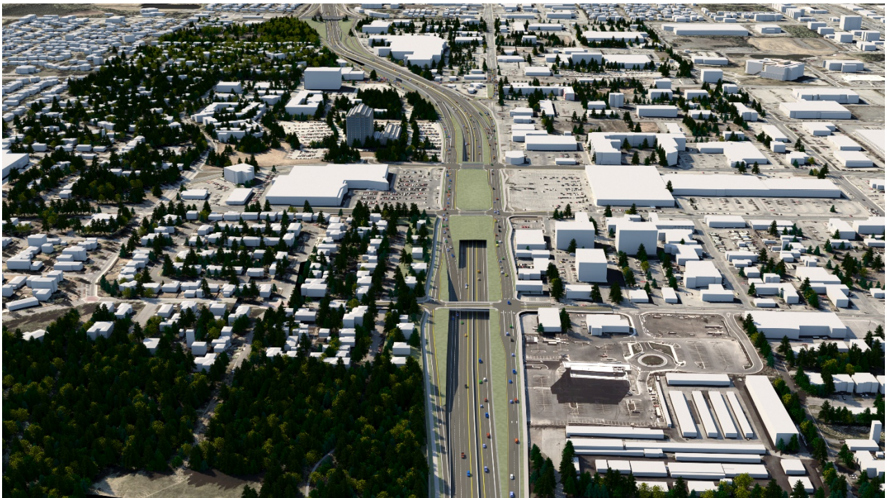
Figure ES-5: Multi-Interchange Concept – Variant 1 (Median U-Turn) looking south with covers over the depressed freeway section
